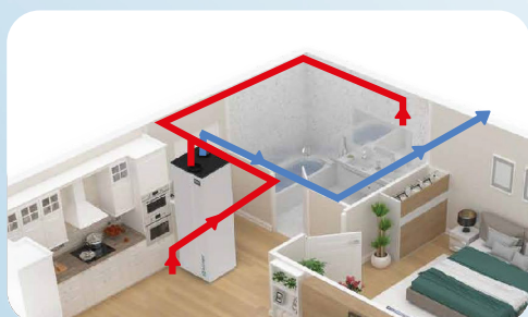
Internal air intake MEV
