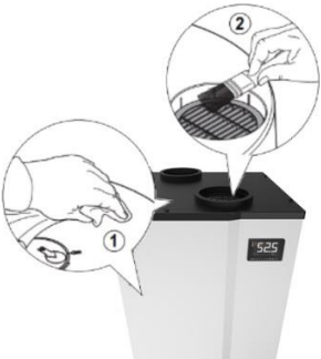
Illustration 16: Maintenance cleaning of the ECOHEAT
