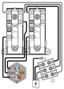
**Electrical connection, diagram - STANDARD** 7.5 kW - 3x400V
