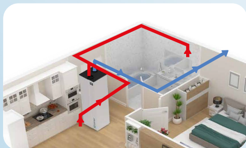
Internal air intake MEV
