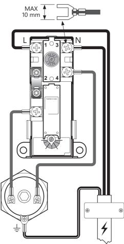
Electric connection, schematic
