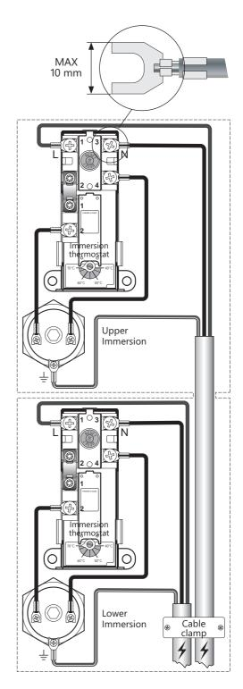
Fork for immersion thermostats (ThermODisc) The unit must be connected to a minimum 16 amp dedicated permanent supply complying with current IET Wiring regulations, isolation is required via a minimum 20 amp double pole isolation switch with a minimum 3 mm separation required. All electrical wiring should be carried out by a competent electrician, using a heat resistant Flexible cable (minimum 90°C), and be in accordance with the latest IET Wiring Regulations.
