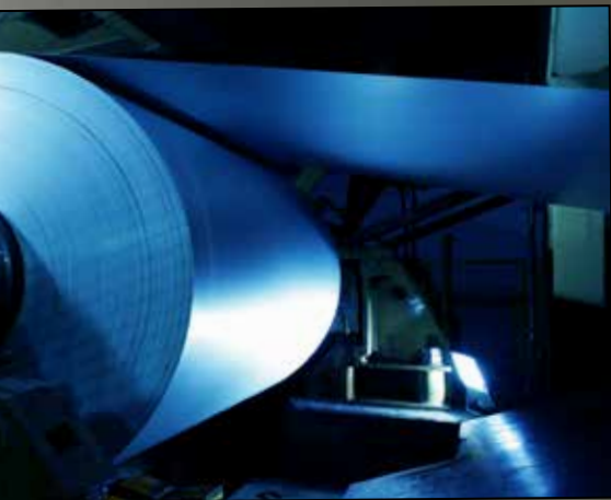
Stainless steel roll feeding spiral weld
