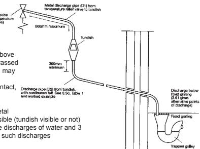
Where a single pipe serves a number of discharges, such as in blocks of flats, the number served should be limited to not more than 6 systems so that any installation discharging can be traced reasonably easily. The single common dis-charge pipe should be at least one pipe size larger than the largest individual discharge pipe to be connected. For further information contact your Building Control Office
