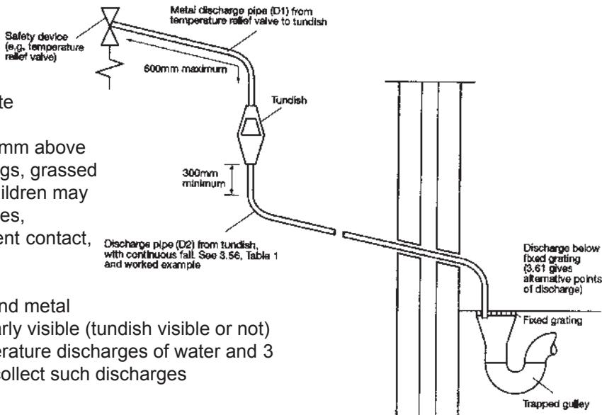
Where a single pipe serves a number of discharges, such as in blocks of flats, the number served should be limited to not more than 6 systems so that any installation discharging can be traced reasonably easily. The single common discharge pipe should be at least one pipe size larger than the largest individual discharge pipe to be connected. For further information contact your Building Control Office
